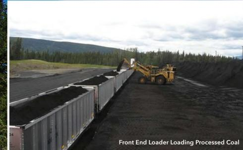
Front End Loader Loading Processed Coal
