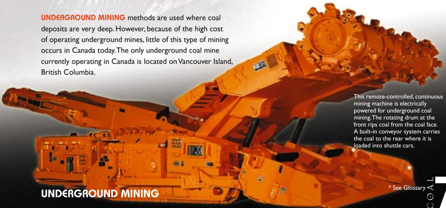
This remote-controlled, continuous mining machine is electrically powered for underground coal mining. The rotating drum at the front rips coal from the coal face. A built-in conveyor system carries the coal to the rear where it is loaded into shuttle cars.
